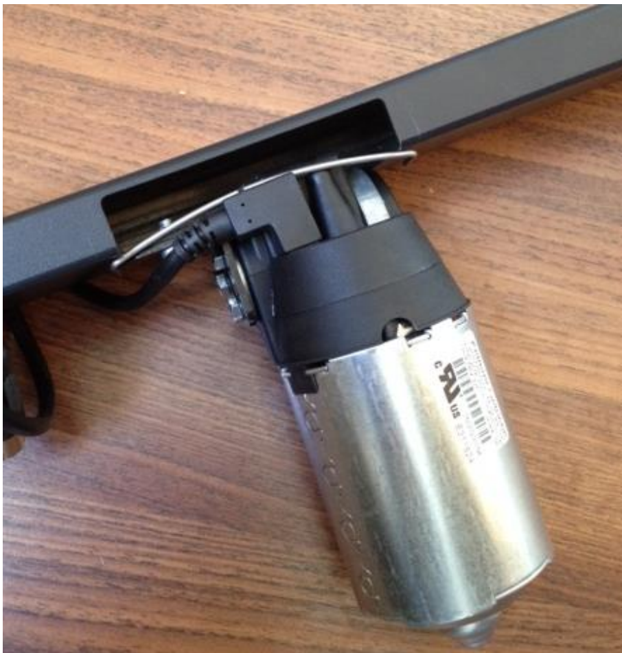
6.1.3 Mount the spring for retention of motor plug.
