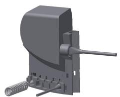
When all cables have been connected, use the safe locking bracket. Pushed in until you hear a "click".
