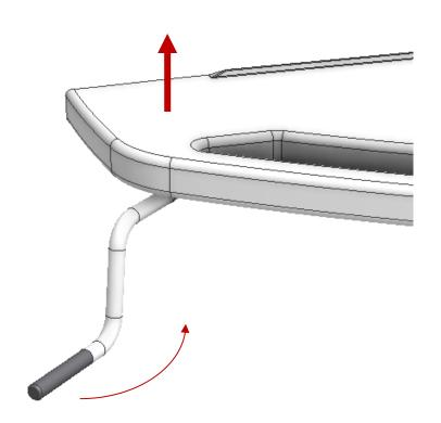
Tip: Move washbasin to top position to facilitate further mounting
