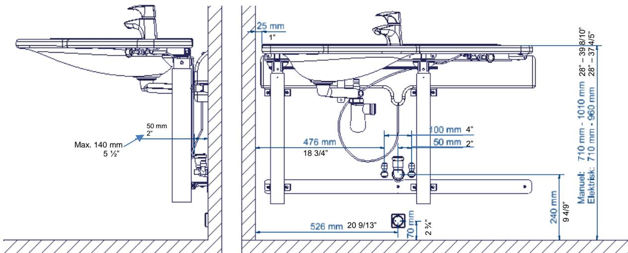
Manual/electrical height adjustment, plumbing located behind the cover.
