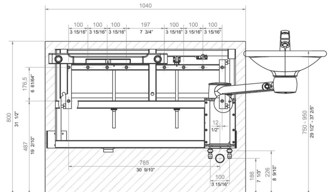
**NOTE:**All dimensions are based on adjustment of the washbasin from 750 - 950 mm (29 ½" – 37 2/5") above floor level. If a change of this height-adjustment range is required, the recommended dimensions must be changed accordingly.
