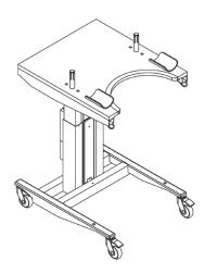
Electric height adjustment 75-135cm. Tabletop 79x68cm in colour light grey with black edges incl. boomerang  $\emptyset$  40cm., hand control, arm supports, handles and 4 pcs. brake wheels.
